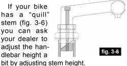
A guill stem has an etched or stamped mark on its shaft which designates the stem's "Minimum Insertion" or "Maximum Extension". This mark must not be visible above the headset.
