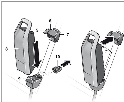
In order for the battery pack to be inserted, the key **5** must be inserted into the lock **6** and the lock must be unlocked.
