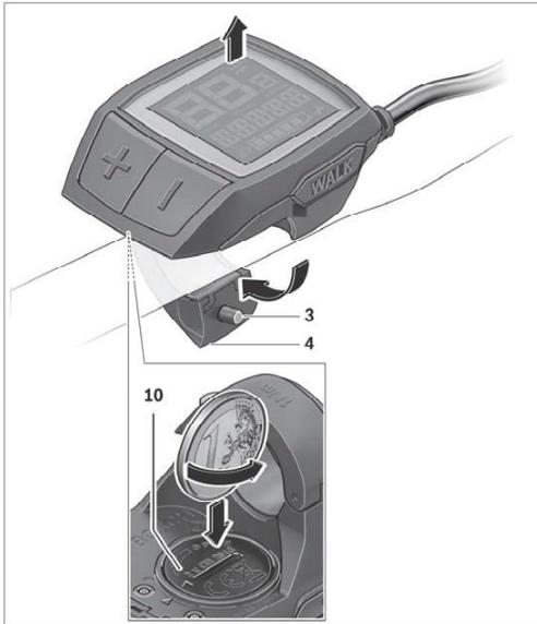
If the on-board computer shows “LOW BAT” on the display, remove the on-board computer from the handlebars by unscrewing the fastening screw **3** of the on-board computer. Open the battery lid **10** using a suitable coin, remove the used batteries and insert new CR 2016 batteries. You can obtain the batteries recommended by Bosch from your eBike dealer.
