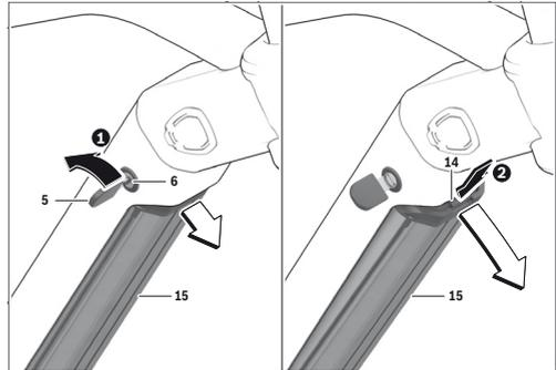
❶ To remove the PowerTube battery, **15** open the lock **6** using the key **5**. The battery will be unlocked and fall into the safety restraint **14**.
