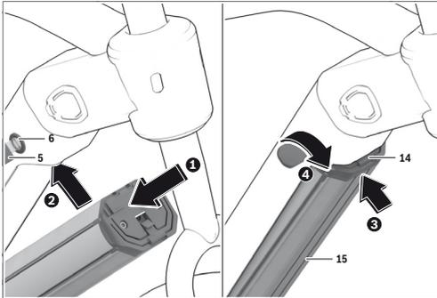
In order for the battery pack to be inserted, the key **5** must be inserted into the lock **6** and the lock must be unlocked.
