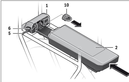
In order for the battery pack to be inserted, the key **5** must be inserted into the lock **6** and the lock must be unlocked.
