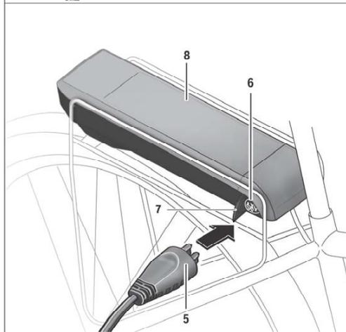
Switch the battery off. Clean the cover of the charge socket 7. In particular, prevent the charge socket and the contacts from getting dirty, e. g., with sand or soil. Lift the cover of the charge socket 7 and plug the charge connector 5 into the charge socket 6.
