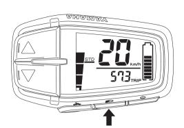
○ Headlight "On/Off" (Applies only to models equipped with a headlight powered by the battery pack. The taillight, which is powered by the battery pack, is switched on/off with the headlight.)
