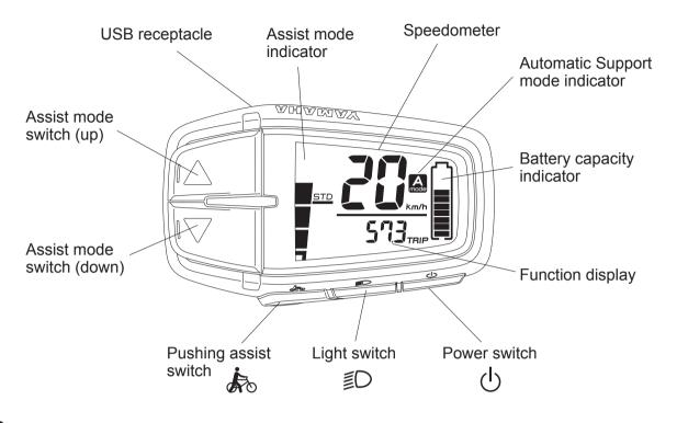
The USB receptacle is for connecting the designated YAMAHA tool; it cannot be used as a power supply.
