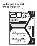
The Automatic Support mode, which enables automatic change to the optimal assist mode according to the riding conditions, can also be used.
