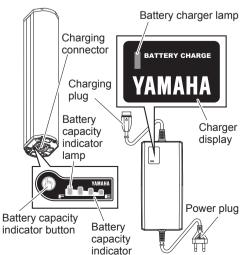
The battery pack equipped for the Yamaha e-Bike Systems is a lithium-ion battery. The lithium-ion battery is lightweight and offers superior capacity. However, it does have the following characteristics.
