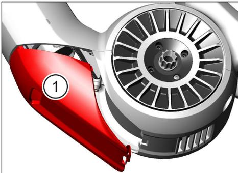
Fig. 10: Removing the SkidPlate
