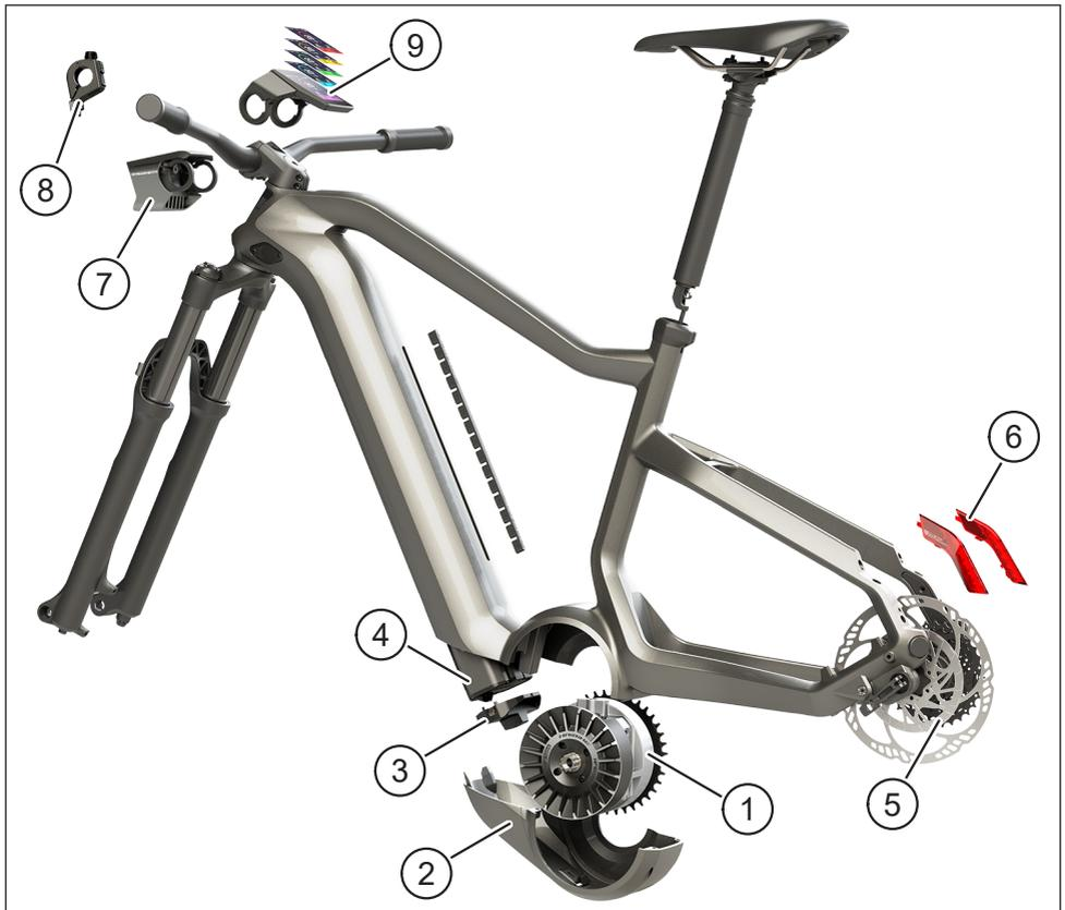
Fig. 1: Components of the FLYON drive system
