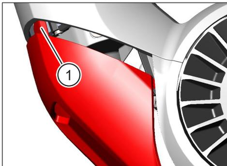
Fig. 19: Lugs on the SkidPlate
