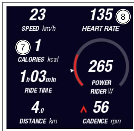
Fig. 36: Training screen with profile and heart rate monitor
